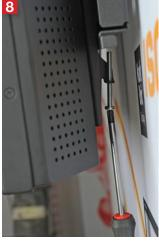
Lock the screen with the two screews in the bottom of the screen rails!
